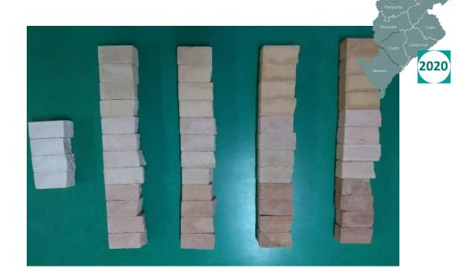
Plastic feature: mortar shades obtained through calcination using iron miner's tailings, with no addition of dyes.
