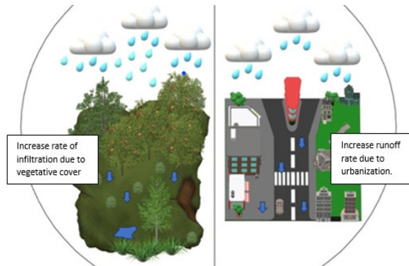
Figure 1.2: Rate of infiltration on a greenfield site compared to urbanized site.
