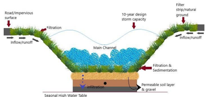
Figure 3.2: Reproduction of a Vegetative Swale. (Ekka et al, 2020)
