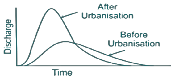
Figure 3.4: Predevelopment discharge rate compared to the post development discharge rate (Simplified Civil, 2022).
